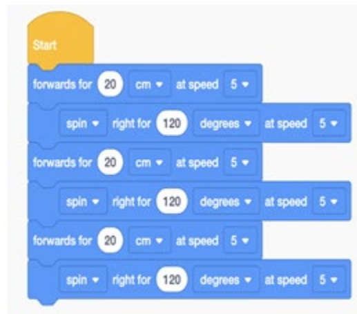
Figure 2 EdScratch Program Designed for an Equilateral Triangle Construction
