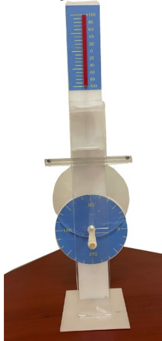
Figure 8 Isolated Rod-and-Cam Section of Wave Machine
