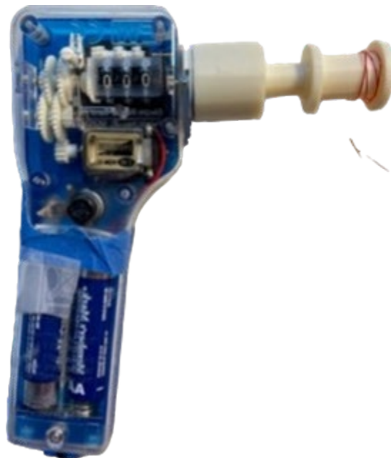
Figure 7 Winder Used to Wrap Wire Around a Solenoid Tube
