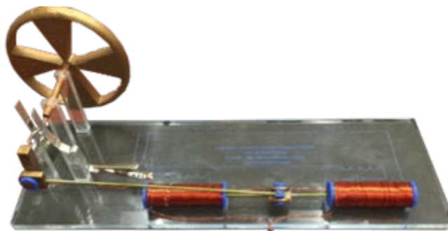
Figure 2 Reconstruction of the Charles Page Engine
